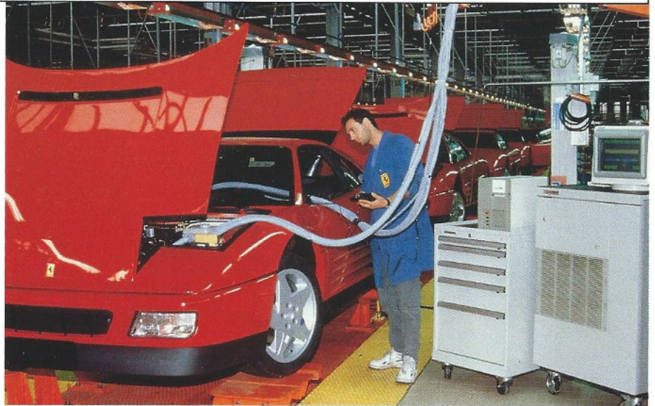
A Ferrari craftsman uses HP test equipment, located at four of 20 Ferrari work sites, to test the electrical system of the newest Ferrari sports coupe.
